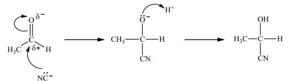
curly arrow going from lone pair/negative charge on C in NC<sup>-</sup> to carbonyl C; curly arrow going from C=O to O; *Do not allow curly arrow originating on N of NC*<sup>-</sup>.
